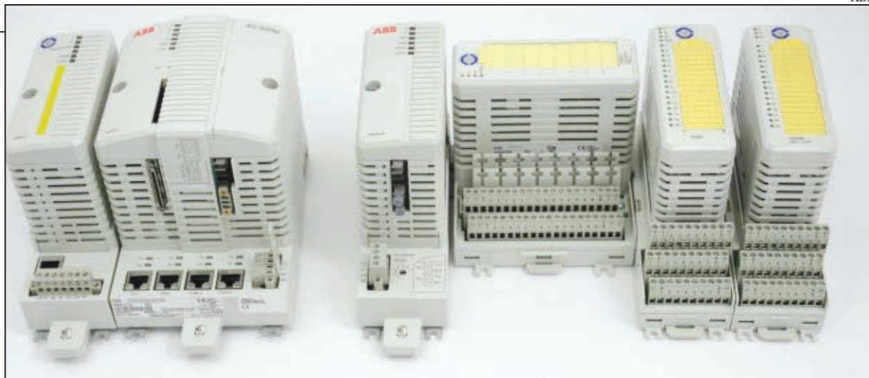
FIGURE 2. ABB's High Integrity safety system, which is paired with its System 800xA for process control, is integrated but separate thanks to "embedded diversity," which means the hardware and software architecture of the controllers is different to ensure that the failure modes of the safety system are completely unique from the potential failure modes of the process control system
