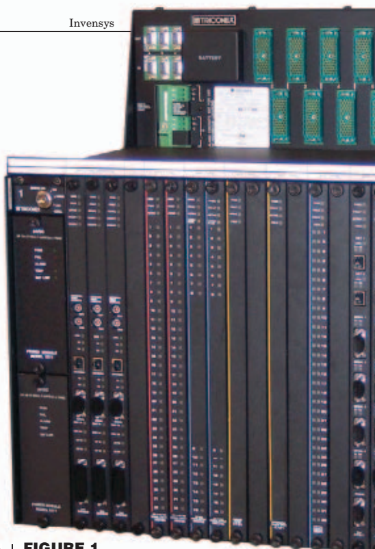
FIGURE 1. This image shows the Triconex Safety Instrumented System configuration from Invensys, with triple modular redundant controllers, input/output modules and communications subsystems
